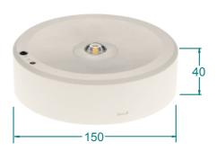
**Specification:** Stand-alone self-contained emergency LED downlight. Constant emergency light (1.5W/150Im & 3W/270Im) for 3 hours. Low stand-by power consumption (0.5W). Self-test versions and remote controls available. Lithium battery integrated. Non-maintained configuration. Ceiling surface mount. Suitable for open area and corridor indoor applications.
