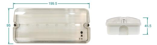
**Specification:** Weatherproof (IP65) and robust (IK10) self-contained and self-test emergency LED bulkhead. Constant emergency light (1.5W/170Im) for 3 hours. Low stand-by power consumption. Remote control available.Self-adhesive legend available for 18m viewing distance exit sign. Lithium battery integrated. Maintained or non-maintained configurations. Suitable for indoor and outdoor applications such as car parks, distribution centres, storage rooms and sports centres.
