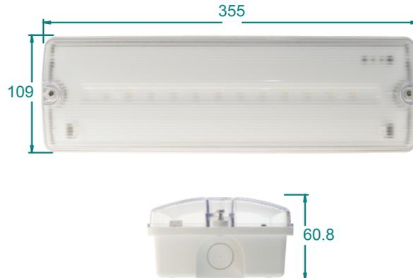
**Specification:** Weatherproof (IP65) and robust (IK10) self-contained emergency LED bulkhead. Constant emergency light (1.5W/170lm & 3W/320lm) for 3 hours. Low stand-by power consumption. Self-test versions and remote controls available. Self-adhesive legend available for 20m viewing distance exit sign. Lithium battery integrated. Maintained or non-maintained configurations. Suitable for indoor and outdoor applications such as car parks, distribution centres, storage rooms and sports centres.
