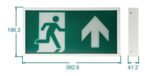
**Specification:** Slim self-contained emergency LED exit sign box. Viewing distance 34m. Constant emergency light (90lm) for 3 hours. Low stand-by power consumption. Self-test versions and remote controls available. Lithium battery as standard. Maintained or non-maintained configurations. Suitable for indoor applications such as educational and offices buildings.
