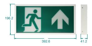
**Specification:** Slim self-contained emergency LED exit sign box. Viewing distance 34m. Constant emergency light (70lm) for 3 hours. Low stand-by power consumption. Self-test versions and remote controls available. Lithium battery as standard. Maintained or non-maintained configurations. Suitable for indoor applications such as educational and offices buildings.
