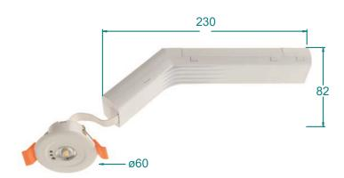
Specification: DALI-2 certified, addressable, stand-alone self-contained emergency LED downlight. Integrated open area, corridor and spot lens. Constant emergency light (3W/325lm) for 3 hours. Low stand-by power consumption (0.5W). Self-test versions and remote controls available. Lithium battery as standard. Non-maintained configuration. Ceiling recessed mounting. Suitable for open area, corridor and spot indoor applications.
