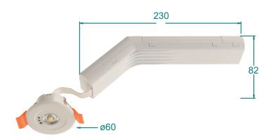
Specification: Stand-alone self-contained emergency LED downlight. Integrated open area lens. Constant emergency light (3W/325lm) for 3 hours. Low stand-by power consumption (0.5W). Self-test versions and remote controls available. Lithium battery as standard. Non-maintained configuration. Ceiling recessed mounting. Suitable for open area and corridor indoor applications.
