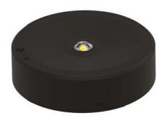
**Specification:** Stand-alone self-contained emergency LED downlight. Corridor lens integrated. Constant emergency light (1.5W/190lm) for 3 hours. Low stand-by power consumption (0.5W). Self-test versions and remote controls available. Lithium battery as standard. Non-maintained configuration. Ceiling surface mount. Suitable for open area and corridor indoor applications.
