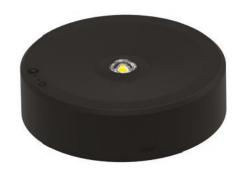
Specification: DALI-2 certified, addressable, stand-alone self-contained emergency LED downlight. Corridor or Open Area lens integrated. Constant emergency light (1.5W/190lm & 200lm) for 3 hours. Low stand-by power consumption (0.5W). Self-test versions and remote controls available. Lithium battery as standard. Non-maintained configuration. Ceiling surface mount. Suitable for open area and corridor indoor applications.
