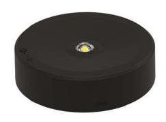
**Specification:** Stand-alone self-contained emergency LED downlight. Open area lens integrated. Constant emergency light (1.5W/200lm) for 3 hours. Low stand-by power consumption (0.5W). Self-test versions and remote controls available. Lithium battery as standard. Non-maintained configuration. Ceiling surface mount. Suitable for open area and corridor indoor applications.
