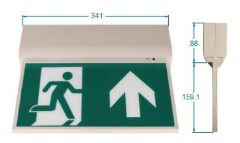
Specification: Double sided self-contained emergency LED exit blade sign. Viewing distance 30m. Constant emergency light for 3 hours. Low stand-by power consumption. Self-test versions and remote controls available. Lithium battery as standard. Maintained, Switch Maintained or non-maintained configurations. Ceiling or recessed mounts. Suitable for indoor applications such as educational and office buildings.
